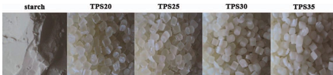
Figure 1 Thermoplastic starch granules. [Color figure can be viewed in the online issue, which is available at wileyonlinelibrary.com .]
